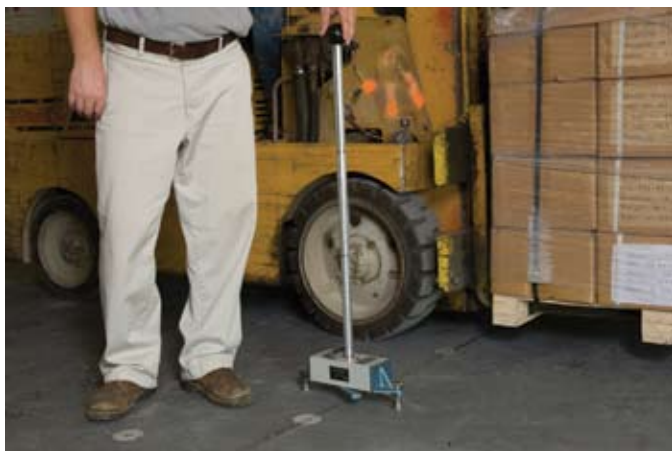
Fig. 3: The relative deflection of the two sides of each joint was obtained using an electronic inclinometer while the wheel of a forklift crossed the joint
